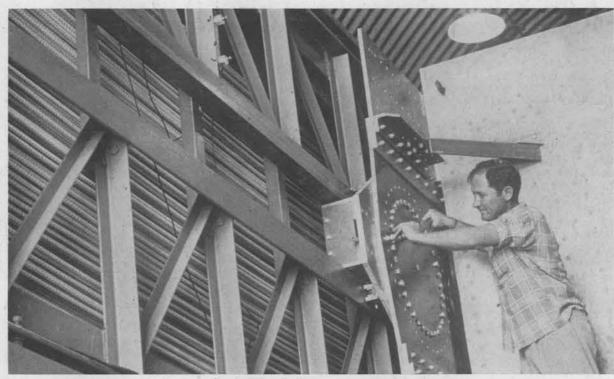
TWO BANKS of shock cords supply the power for acceleration tests in the new "Slingshot" test in-
